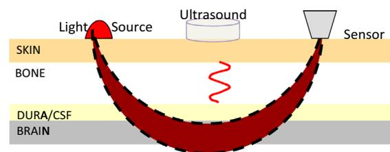
**Fig 4. Schematic of US-tagged NIR device,** in which light source indicates laser NIR, ultrasound indicates integral ultrasound crystal incorporated into the device and imparting Doppler shift to NIR light, sensor represents sensing component of UTLight Flowmetry NIR device, and skin, bone, dura/CSF and brain represent various tissue layers.
